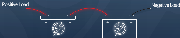
Series Connection 24V 100Ah Bank Increases Voltage, Ah stays the same.
