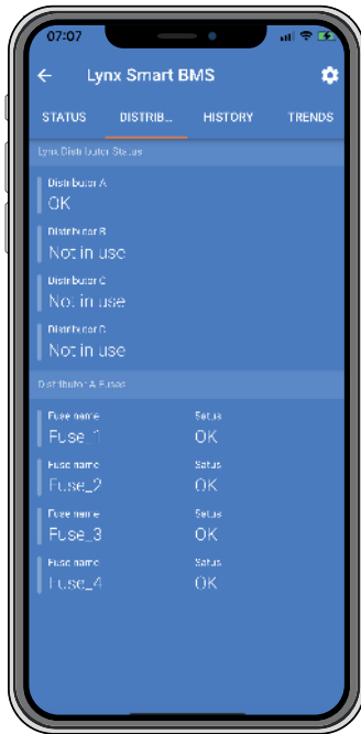
The VictronConnect App Lynx Smart BMS showing Lynx Distributor status
